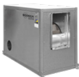
216 CJSRX Extraction units 400 °C/2h to work outside the fire risk zone, driven by transmission with a backward curved impeller
