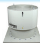
Roof-mounted axial extractor fans with vertical air outlet, ATEX Certification and possibility of Ex e, Ex d, Ex tc and Ex tb marking
